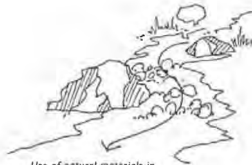
Use of natural materials in man-made drainage channel.
